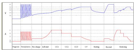
Stage 1 - Diagnosis: Analyze if the battery can accept a charge or not, and then prevent charging from proceeding on the a defective battery;
